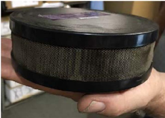
Example of a dirty filter that must be changed for a new filter. Continued use of a filter in this condition will stress the blower motor and may lead to a violation of the warranty.
