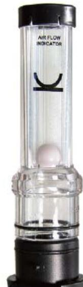
Example of airflow below 170LPM. Inspect and change HEPA if necessary.
