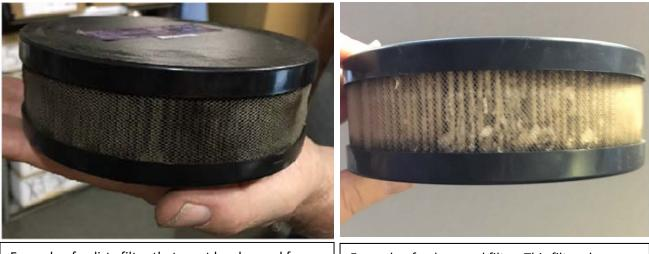
Example of a dirty filter that must be changed for a new filter. Continued use of a filter in this condition will stress the blower motor and may lead to a violation of the warranty. Example of a damaged filter. This filter shows signs of physical damage. Misuse of the filter voids the warranty.
